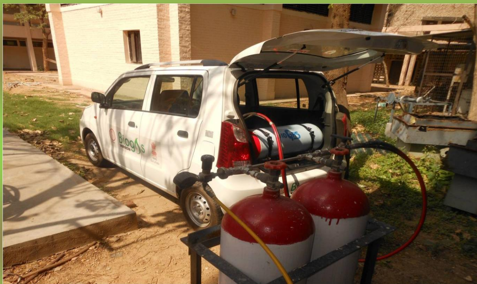
Bio-CNG Filling in biogas fuelled passenger car at Enrichment and Bottling Laboratory, IIT Delhi
